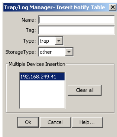
Figure 103 Insert Notify Table dialog box for ERS 55xx/35xx and Ethernet Switch devices
