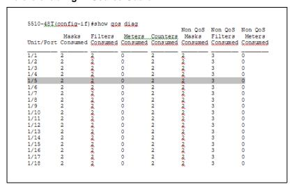
The following figure shows the show gos diag display after enabling IP Source Guard on port 5.
