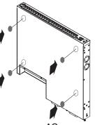
Set the device on a flat surface near an AC power source, making sure there are at least 2 inches (5.1 cm) of space on all sides for proper air flow and at least 5 inches (12.7 cm) at the back for power cord clearance.
